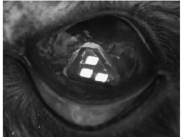
Fig. 1. Fluorescent marker array on the eye of a chinchilla. For this photograph, the eye was illuminated with visible light in addition to UV. Under normal testing conditions, only UV illumination is used, increasing the relative brightness of fluorescent markers.
